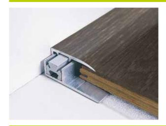
The patented MULTICLIP CLP 270 aluminum perimeter profile allows floor edge finishing without baseboards. A 16mm internal cavity allows 5mm of differential movement. This profile is also suitable along sliding door tracks and as entrance mat framing.
